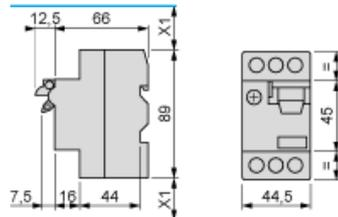
X1: Electrical clearance = 40 mm for  $U_e < 690$  V
