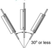
When installing the panel in a slanted position with an incline more than 30 $^{\circ}$ , the ambient temperature must not exceed 40 $^{\circ}$ C (104 $^{\circ}$ F). You may need to use forced air cooling (fan,A/C) to ensure the ambient operating temperature is 40 $^{\circ}$ C or less (104 $^{\circ}$ F or less).
