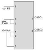
With External Device Monitoring (EDM) feedback loop
