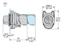
e: clamping thickness: 1 to 6 mm / 0.04 to 0.24 in. (1): Additional row of contacts
