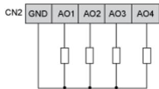
AO3, AO4 can be used also as PWM generator, up to 2kHz.
