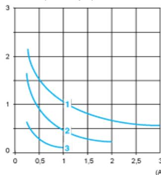
DC-13 Control of electromagnets ( $L/R \leq 2 \times (U_e \times I_e)$  in ms, with  $U_e$ : rated operating voltage and  $I_e$ : rated operating current)
