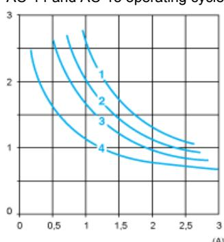
AC-14 Control of weak electromagnetic loads of electromagnets  $\leq 72$  VA (make:  $\cos \phi = 0.3$ , break:  $\cos \phi = 0.3$ )
