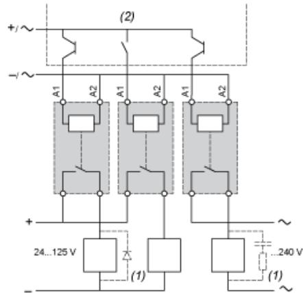
(1) Essential on inductive loads (can be replaced with peak limiter)
