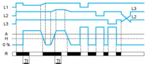
Control of Overvoltage and Undervoltage in Window Mode
