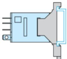
With this mounting type, test button becomes inaccessible
