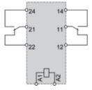
NOTE: For DC input, A1 have to be +, otherwise it would short circuit from protection module
