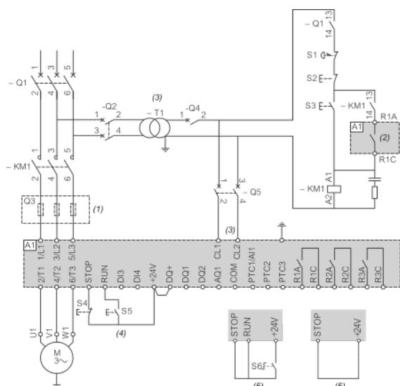
(1) : Installation of additional fast-acting fuses to upgrade to type 2 coordination according to IEC 60947-4-2.
