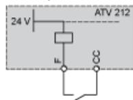
“PLC” position with PLC transistor outputs
