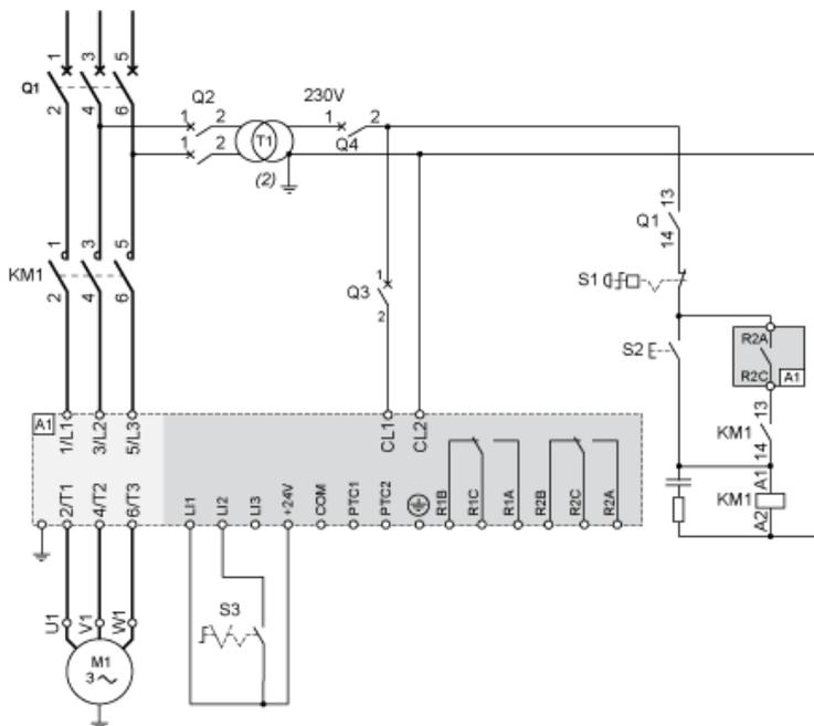
230 Vac control, logic Inputs (LI) 24 Vdc, 3-wire control
