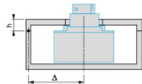
Door cut-outs require a minimum distance between the centre of the circuit breaker and the door hinge point  $\Delta \geq 100 + (h \times 5)$
